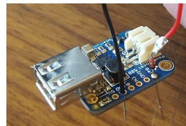
At this point the circuit board should turn on in direct sunlight. There are 2 LEDs on the board. The green LED indicates power. The red LED indicates the input voltage is below 3.2V.
